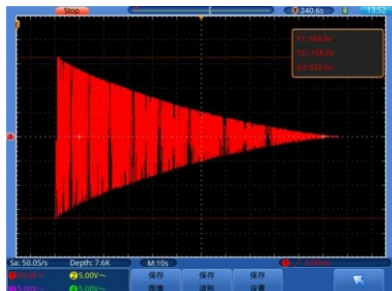
Fig. 6. Measured waveform of load voltage
